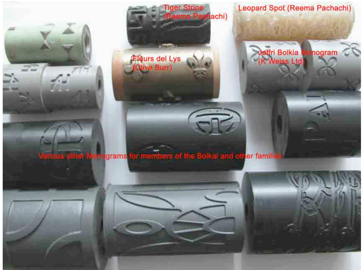
Pattern rollers, mostly made to order for bespoke engine turning designs. The design owners are variously marked where known.
