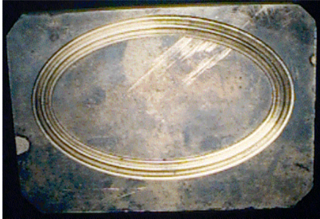
An oval "Moulding" for a picture frame, made by using a series of shaped profile tools This was a gilding metal master pattern for casting from which the inside and outside were to be pierced away leaving just the moulding to be cast as a bezel to fit a frame
